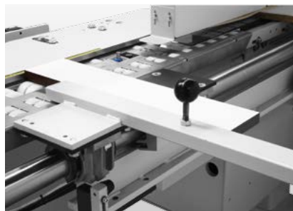
Sliding carriage Robust linear guiding system to secure rectangular workpiece feeding. With EDGETEQ S-380, S-500. Photo = EDGETEQ S-500.
