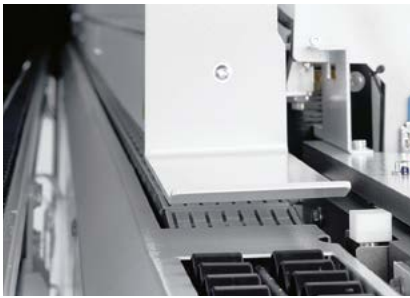
Infeed stop For minimum workpiece spacing and safe operation. With EDGETEQ S-380.
